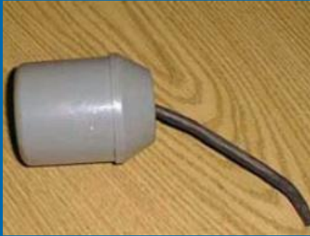
Root Switch from Sump Pump
