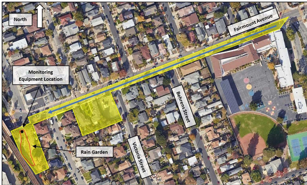
Figure 1. Ohlone Greenway Rain Garden drainage area (yellow) and location of LID facility area (red)
