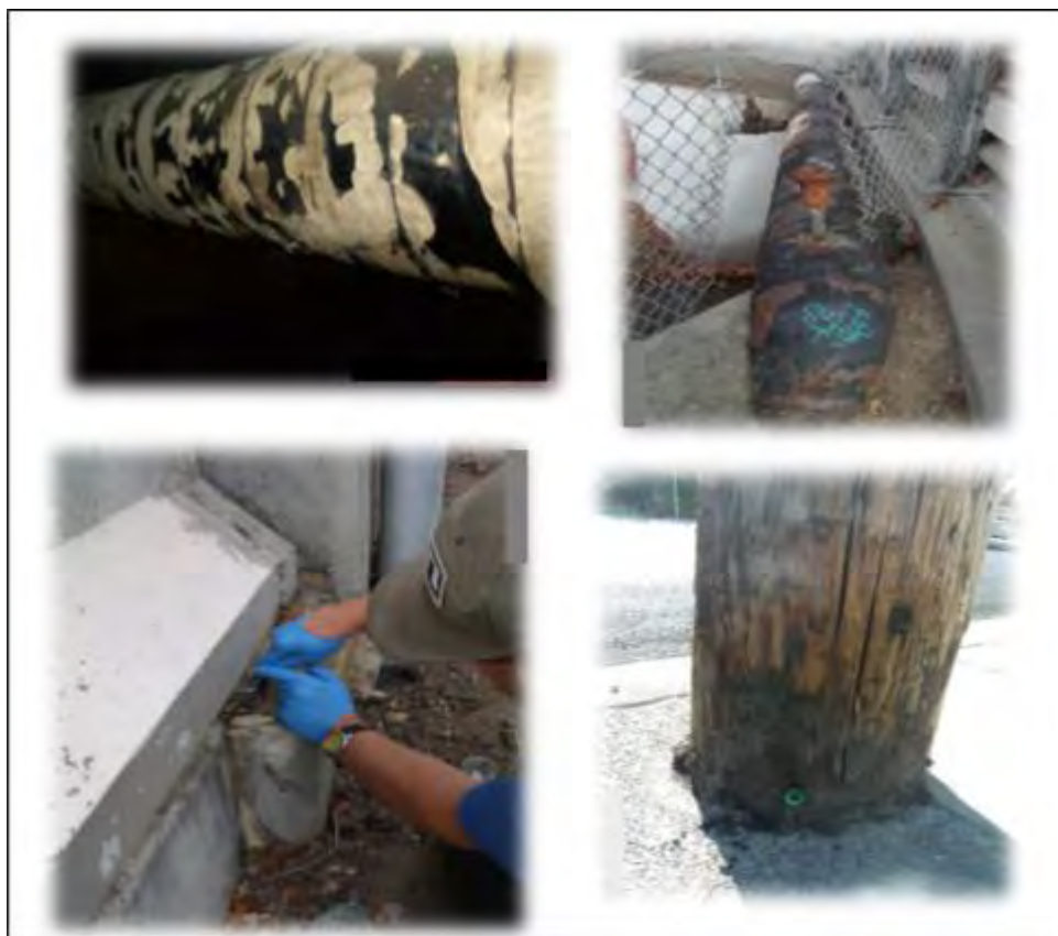
Figure 3.4 Examples of structures that were sampled and sealant materials that were included in the composites that had Moderate PCBs ( \geq 1 ppm and < 50 ppm). Not all structures/samples in the Moderate PCBs category are pictured here.
