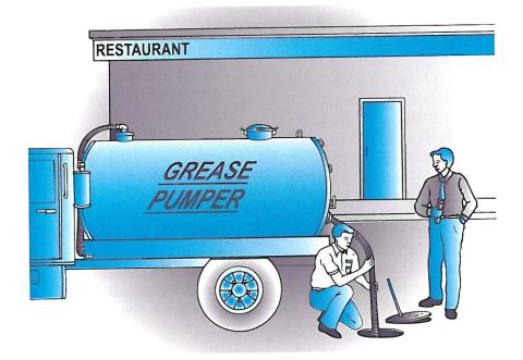
only be connected to a grease interceptor. Eliminating use of a garbage grinder will reduce interceptor cleaning costs.
