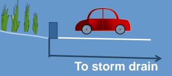
Grade self-retaining areas to drain inward. Set any area drains to pond 3"-4"
