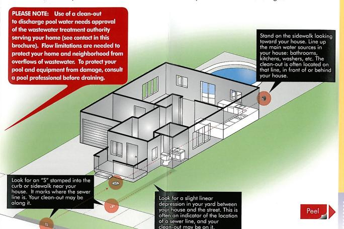
here are a number of places to look for your sanitary sewer clean-out. Start by checking to see if there's an "S" stamped into the concrete of your curb or sidewalk. This marks the location of the sewer line, and your clean-out may be aligned with this marking.
