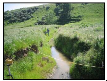
SITE NOTES: Plane-bed channel incised about 5 feet into historic floodplain. Small incipient floodplain forming within channel banks, primarily formed from bank colluvium and downstream transport. Minimal meandering but variable active channel width, primarily due to bank slumping.
